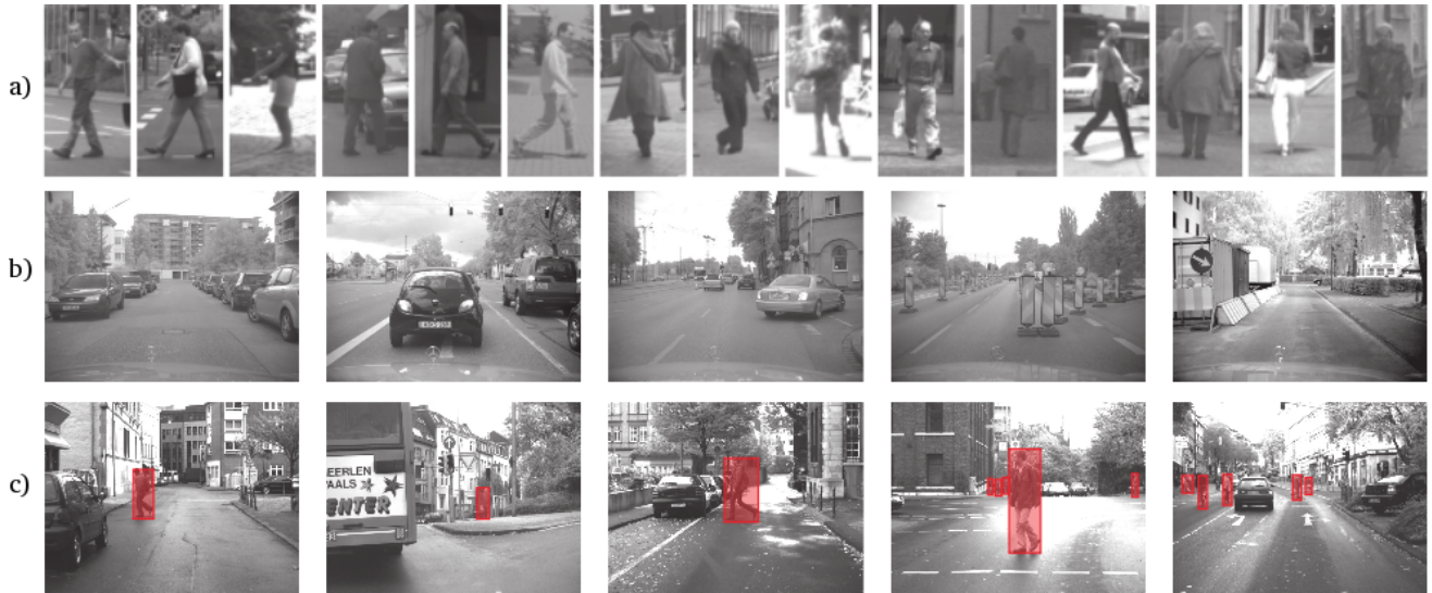
Fig. 5. Overview of the detection benchmark dataset: a) pedestrian training samples. b) non-pedestrian training images. c) annotated test images.
